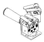
An offset configuration puts the most important controls inline with the user's thumb. The detachable handle permits configuration for left-hand operation.
