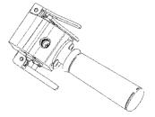
A variation of the threefunction pendant puts one lever underneath the handle. This creates a "trigger," allowing the user to simultaneously work the top control and the bottom control.
